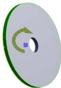
Figure 4 Loads and Supports. Support: Blue highlighted surfaces. Load: Green highlighted surface (see Table 3)
