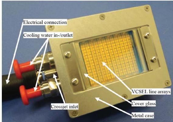
Fig. 5. VCSEL unit of the modular ATP head.
