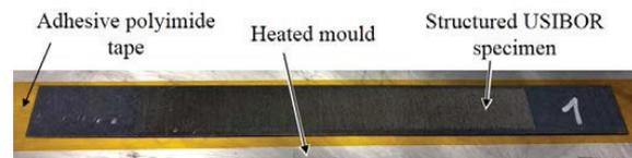
Fig. 4. Metal sample on heatable mould.
