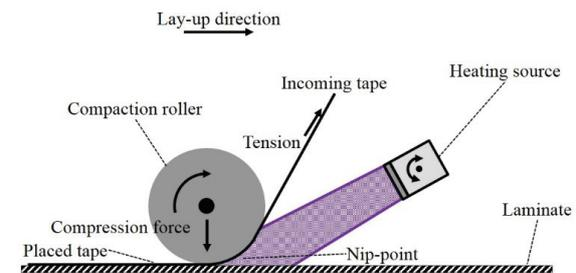
Fig. 2. Principle of an ATP process.
