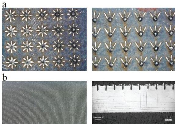
Fig. 1. Different approaches of surface conditioning. (a: Additive structure (Aimen); b: Protruding structure (left: Fraunhofer IPT / right: Fraunhofer ILT)) [16]
