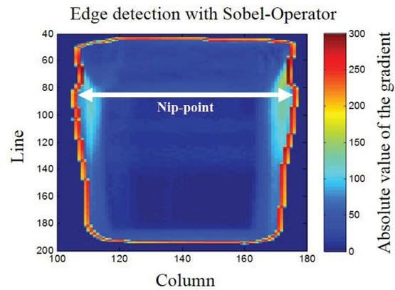
Fig.6. Detection of the position of the nip-point.
