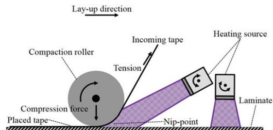
Fig. 3. Two separate heat sources within an ATP head.
